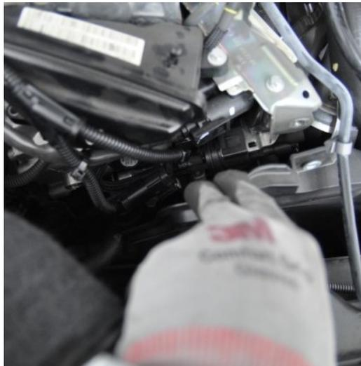
Release the connectors and plug the two wiring harness between the sensor and the original plug.
