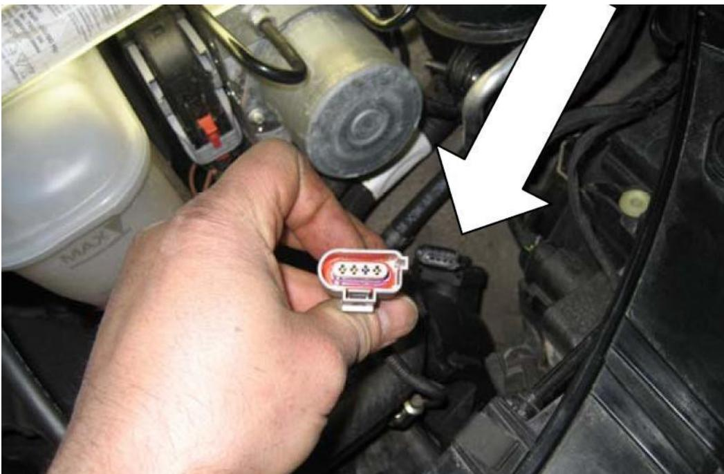
Please make sure during move and attach the cable with cable ties and the SCP module that there is a sufficient distance from parts of the engine (exhaust gas recirculation, turbocharger, exhaust manifold, etc.).
